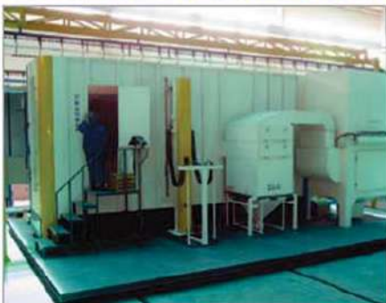
Steel Sheet Surface Coating Automatic (Make- Huali, China) Control Production Line Maximum Size of work piece : L 2400 x W 1000 x H 1500 Powder Coating : Electric Static Spray Conveyor Speed : 3.5m/min (0.5~4.5)m/min adjustable.
