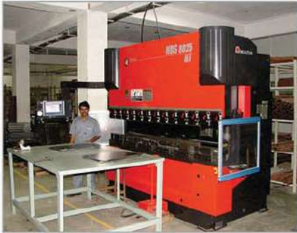
Make- Amada, Japan Capacity - 80 Ton Accuracy - 0.1 mm Working Length - 2600 mm
