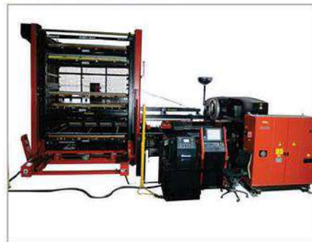
CNC Turret Punch Press (2013) (Make-Amada, Japan) Punching Capacity 20 Tons Punching Accuracy 0.02 mm Working Length 1250 X 2500 mm Maximum Sheet Thickness 3.2 mm
