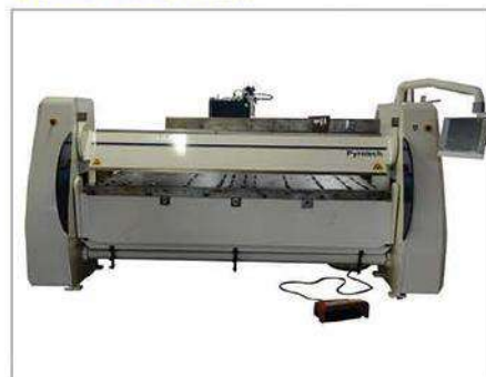
Power Folder Futura Plus-25 (Make- CIDAN, Sweden) Folding Length 2600 mm Capacity at 400 N/sq. mm 3.5 mm Opening Height Clamping Beam 195 mm Motor Clamping Beam 2.2 kv Motor Folding Beam 1.5+1.5 kv Weight Cap.4295 kg
