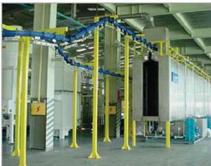
Conveyorized Surface Treatment (Make- Huali, China) Complete surface Treatment which involves processes like Predegreasing, Degreasing, Rinsing 1, DI Water Rinsing 1, NT 1, DI Water Rinsing 2, DI Water Rinsing 3, DI Water Spray.
