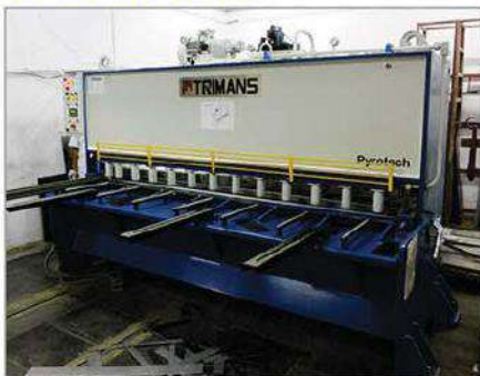
NC Hydraulic Shear Machine (2000) Capacity 4 mm X 3000 mm Work Length 4 x 1000 mm Accuracy up to 0.5 mm Tolerance 0.5 mm
