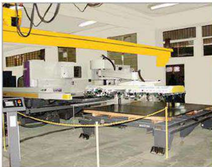
CNC Turret Punch Press (2013) (Make-Muratec, Japan) Punching Capacity 20 Tons Punching Accuracy 0.1 mm Working Length 1250 X 2500 mm Maximum Sheet Thickness 3.2 mm
