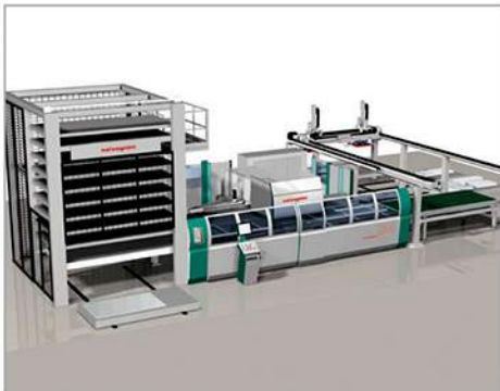
CNC LINE S4 (2013) (Make-Salvagni, Italy) Punching Capacity 20 Tons Punching Accuracy 0.1 mm Working Length 1250 X 2500 mm Maximum Sheet Thickness 3.2 mm
