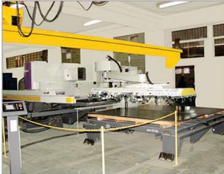
CNC Turret Punch Press (2013) (Make-Murtec, Japan) Punching Capacity 20 Tons Punching Accuracy 0.1 mm Working Length 1250 X 2500 mm Maximum Sheet Thickness 3.2 mm
