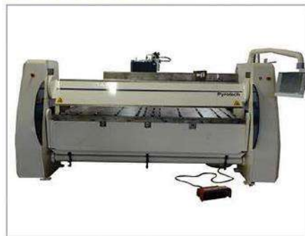
Power Folder Futura Plus-25 (Make- CIDAN, Sweden) Folding Length 2600 mm Capacity at 400 N/sq. mm 3.5 mm Opening Height Clamping Beam 195 mm Motor Clamping Beam 2.2 kv Motor Folding Beam 1.5+1.5 kv Weight ca.4295 kg
