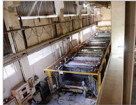
HOT 7 Tank Surface Treatment Capacity 7000 L Provides complete surface Treatment which involves processes like Degreasing, Rinsing, Derusting, Cleaning & Rinsing, Cleaning, Activation, Phosphating, Rinsing, Passivation.
