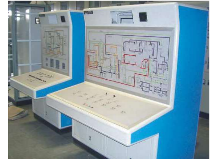
Control Desk and mimic diagrams for power stations on with SMF 48X24 function modules in mixed construction mode with SM 24 mosaic.
